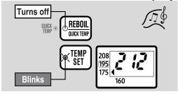
When the boiling process has completed, a melody sounds, the BOIL light turns off, and the KEEP WARM light begins to blink.
