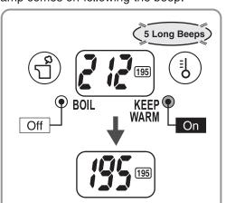
When the temperature reaches 195°F, the temperature shown on the Display will change to 195°F.
