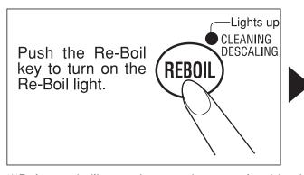
When re-boiling is completed, the Reboil light goes off and the Keep Warm light comes on.
