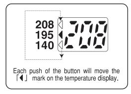
If you want to return to the 208°F Keep Warm set up Push the TEMP SET key and adjust the "  $\P$  " mark on the temperature display to "208°F Keep Warm".
