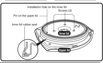
Hot water may leak from the gap between the upper lid and the body when tilted if the inner lid rubber seal becomes old and turns white. This may result in scalds.
