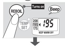
When the Reboil process is completed, the product switches to Keep Warm mode.
