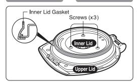
Hot water may leak from the gap between the Upper Lid and the Body when tilted if the Inner Lid Gasket becomes old and turns white. This may result in scalds. If hot water spews from the gap or there is steam even after replacing the Inner Lid Gasket, other parts may be in need of repair. Please contact Zojirushi Customer Service.
