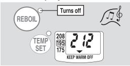
When the boiling process has completed, a melody sounds and the BOIL light turns off.
