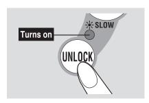
The UNLOCK light turns on and hot water can be dispensed.
