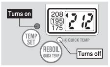
When the boiling process has completed, the BOIL light turns off and the KEEP WARM light turns on.
