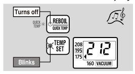
When the boiling process has completed, a melody sounds, the BOIL light turns off, and the KEEP WARM light begins to blink.
