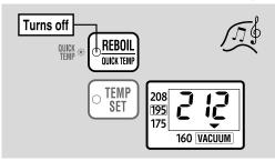
When the boiling process has completed, a melody sounds, and the BOIL light turns off.
