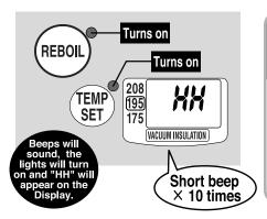
Be careful not to repeat the boiling process without filling the Inner Container with water, as the Nonstick Coating may discolor and peel. The Automatic Shut-Off function activates to shut down power to the heater in order to prevent damage from overheating. The Display will show "HH" to alert you that the Automatic Shut-Off has been activated. The following conditions may cause activation:
