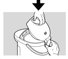
Hold the product with both hands and dispose water where indicated "EMPTY FROM HERE" on the wall of the Inner Container.
