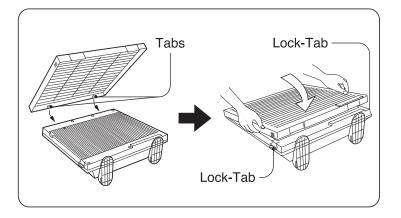
5 Return the Air Purifier to upright position and plug the Power Plug into an electrical outlet.
