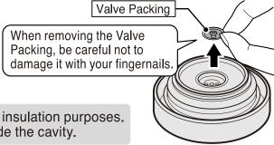
• The Lid Set has a hollow structure for insulation purposes. Remove the Lid Cover and clean inside the cavity.
