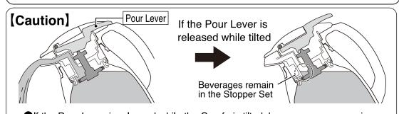
●If the Pour Lever is released while the Carafe is tilted, beverages may remain in the Stopper Set and cause leaks while in use, resulting in burns or stains.
