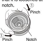
②Pinch the Stopper Packing at the notch and remove the Stopper Packing.
