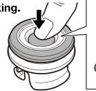
Please make sure to fit the Valve Packing in the center hole.
