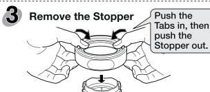
Push the Tabs on the Stopper in toward the center to remove the Stopper. (Lining up the Tabs on the Stopper with the > < marks will make the Stopper easy to remove.)
