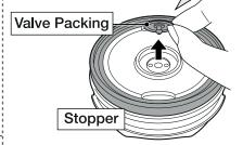
The Valve Packing is fitted in the center of the Stopper. Remove it using finger and thumb as shown in the illustration.
